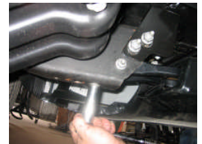
Fig 4 Pass side Tow Hook Bolts and Frame Horn Nuts
