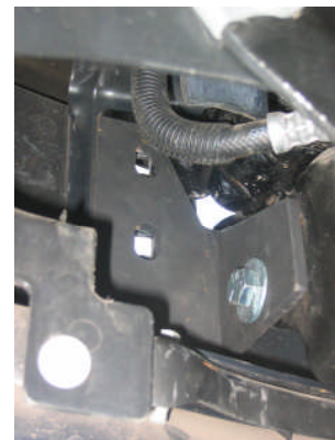
Fig 3. Close up of Driver's side Stiffener bracket attached to the frame
